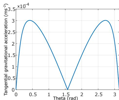
Figure 16: Tangential acceleration at the surface of an ellipse
