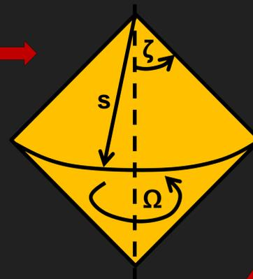
**Gravity field of a double-cone top:** The gravitational *potential* for a circular lamina is standard and is available in [1]. We numerically integrate the same along the height of the cone. For a disc of radius  $a$  at a height of  $z$  from the center of the cone, the formula for gravitational potential  $\varphi_{disc}(\mathbf{r}, a)$  at any point with position vector  $\mathbf{r} (= R\mathbf{e}_r + Z\mathbf{e}_k)$  not on the disc is given as,
