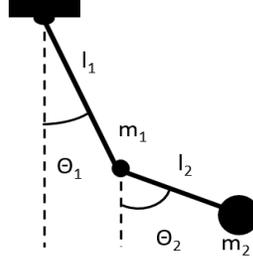
Figure 4: Double pendulum schematic diagram
